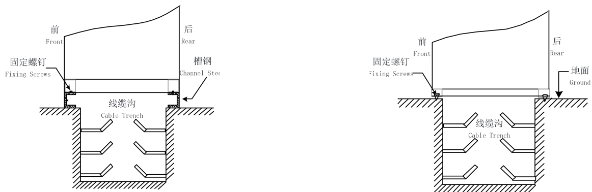
(a) Schematic diagram of the equipment fixed to the channel (b) Schematic diagram of the equipment fixed to the ground
